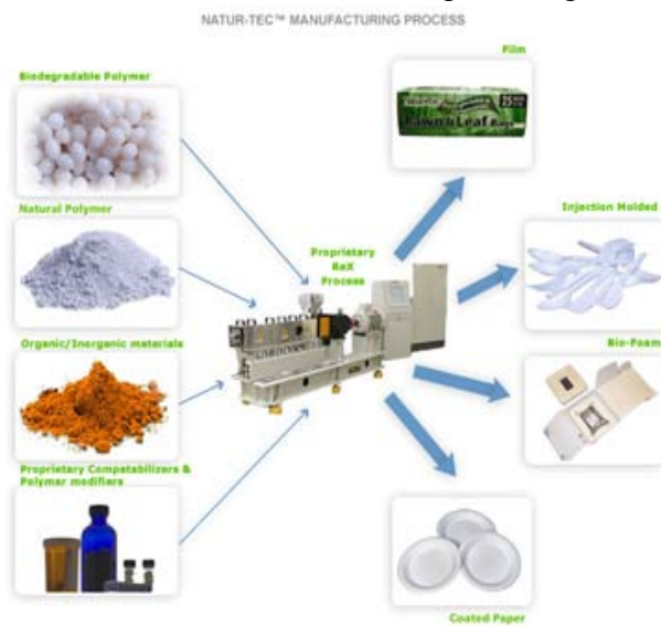
Figure 2.1.1: Raw materials used for biodegradable plastic production. Source: Natur-Tec Sustainable Biobased Materials.
